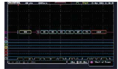
CAN Bus Trigger and Decode
