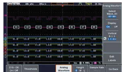
Display analog waveform converted from digital signal
