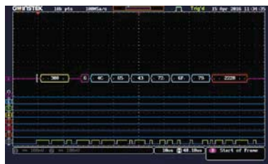
Decode by digital Channel
