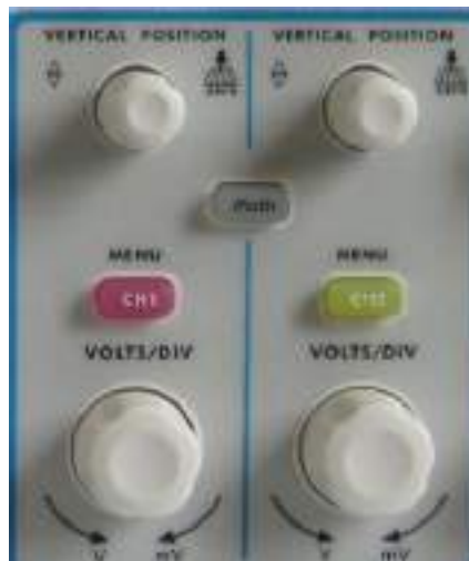
Fig. 4-12 Vertical Control Zone
