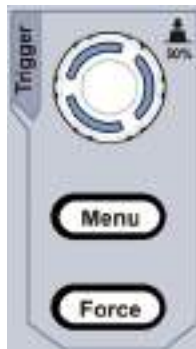
Figure 3-12 Trigger Control Zone
