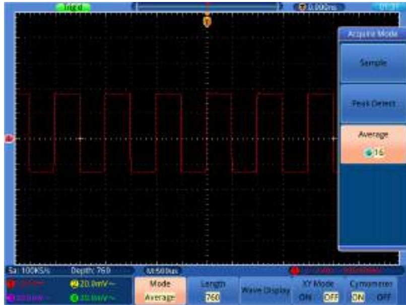
Figure 7-5 Reduce Noise level by using Average function
