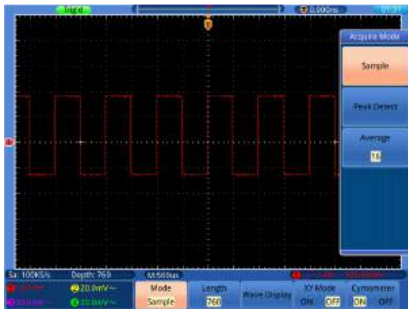
Figure 5-3 Normal ACQU Mode display, in which no burr can be detected.
