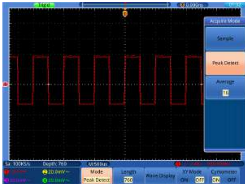
Figure 5-2 Peak Detect mode, under which the burrs on the falling edge of the square wave, can be detected and the noise is heavy
