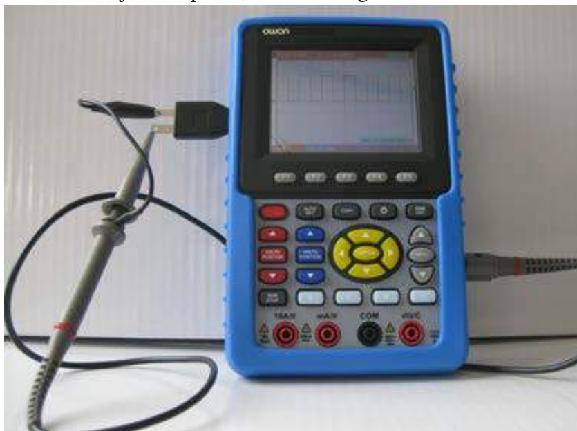
Fig.3. The connection of Square-wave test signal
