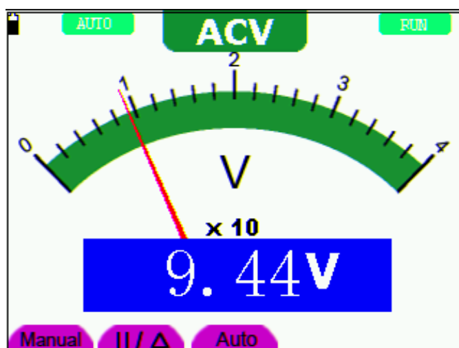
Figure 26: AC Voltage Measurement
