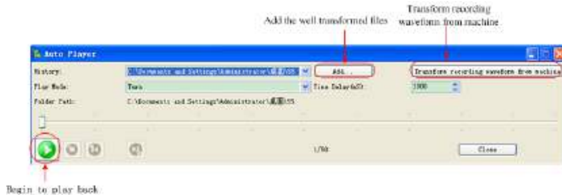
Figure 4-17: Play back waveform by software
