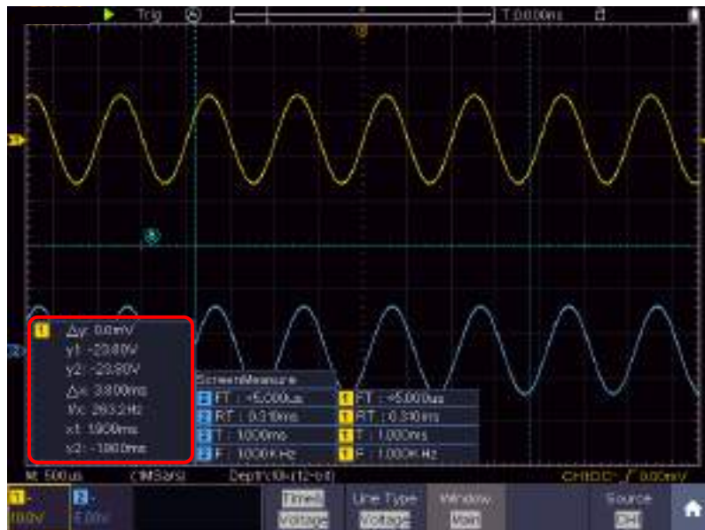
Figure 4-21 Time&Voltage Cursor Measurement
