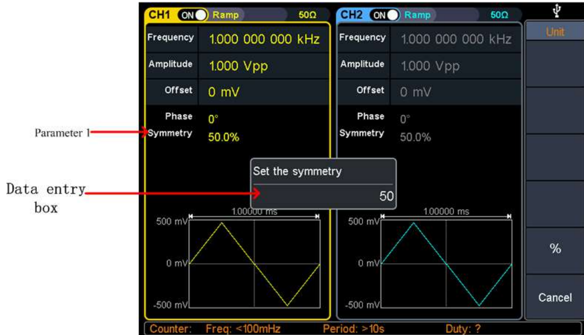
Figure 5-5: Set the symmetry of ramp wave
