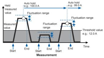
If the measured value falls below the threshold value (voltage, current) or exceeds the threshold value (resistance, continuity, diode) after display value updates are stopped, display value updates will stop once more if the two conditions are satisfied again.
