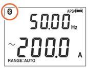
icon will flash when the instrument is connected to a mobile device.
