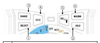
Selects alternate measurement modes on a rotary switch setting, including:
