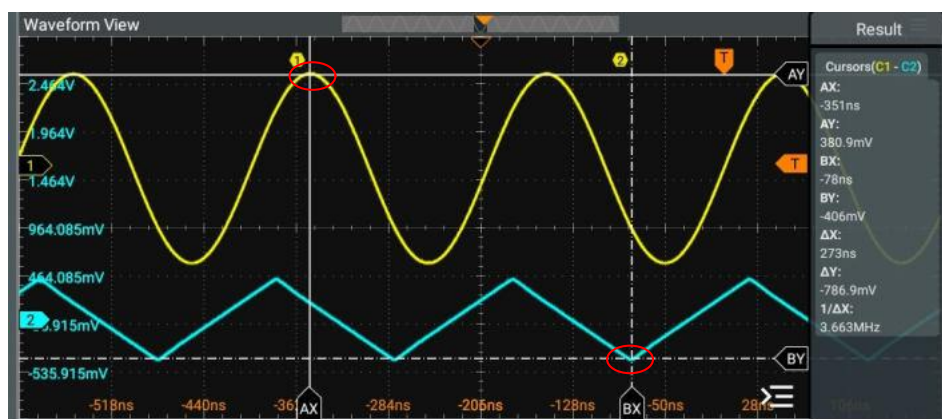
Figure 10.13 Track Measurement (after Horizontal Expansion)
