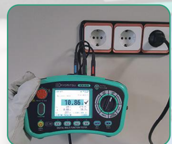
Loop test from a wall socket
