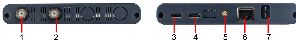
Figure 3-2. Communication Interface of the Device
