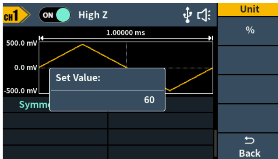
Figure 5-6: Set the symmetry of ramp wave
